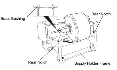
**2.** Now feed the media from the bottom of the media roll into the media slot at the rear of the printer as shown.
